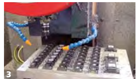
3 Picture 3. The use of a multiple workholding system is also beneficial in small batch machining
